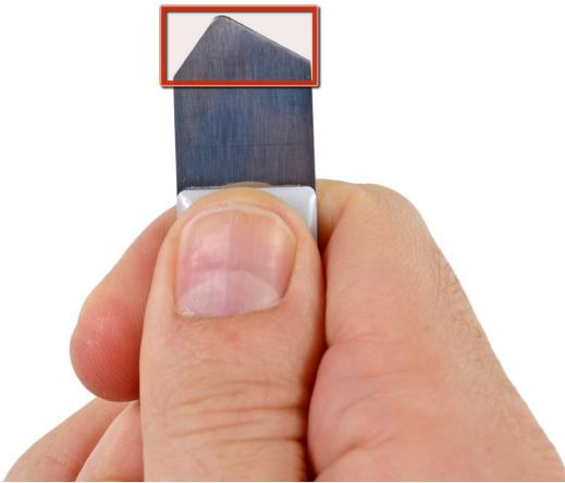
**i** In the following steps, you will use the iSesamo tool to detach the adhesive holding the front glass to the aluminum frame of the iPad 3.
